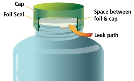
Bottle with cap loosened (de-torqued)
