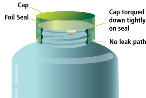
Bottle with cap tightly closed (fully torqued)
