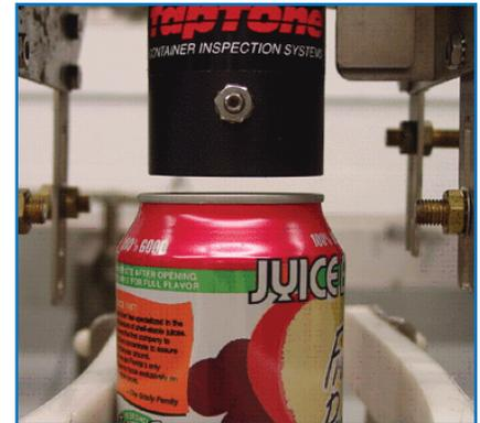
A can of juice passes underneath the proximity sensor.
