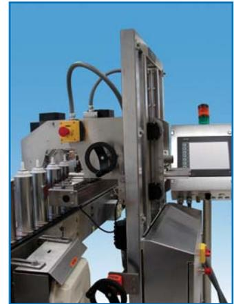
Cans of aerosol whipped cream being tested in the TapTone 4000-FS Force System
