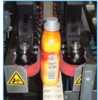
A bottle of fabric softener passes through the compression belts of the T1000-C.
