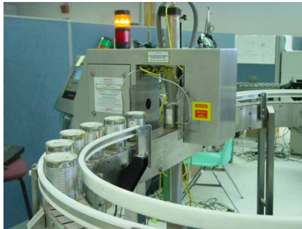
▲ Cans are tested with the T500 x-ray sensor.
