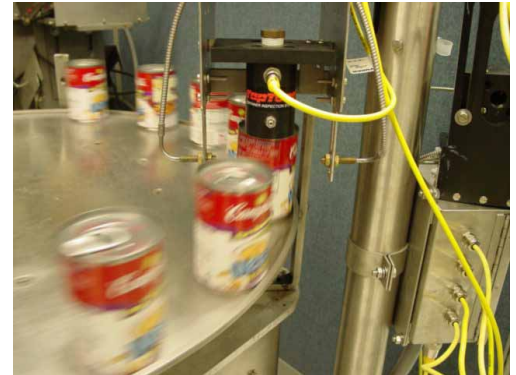
▲ EZ open soup cans are tested with the T500-P.
