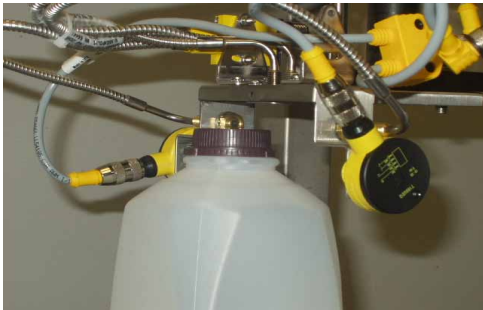
▲ Containers being inspected on the process line with the dual bifurcated missing cap assembly.
