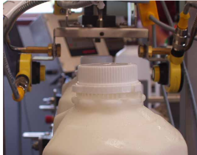
▲ Containers being inspected on the process line with the dual bifurcated missing cap assembly.
