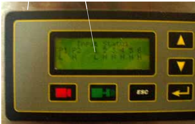
▲ For the missing cap application we used Input (1) one as the port. With the system set-up correctly we can monitor the status of the option. When a good container with a lid passes by the inspection bridge we can expect a low signal every time.
