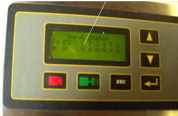
▲ When a container with a missing lid is presented to the inspection bridge the signal for input (1) one will go high. Then the container will be rejected from the production line.
