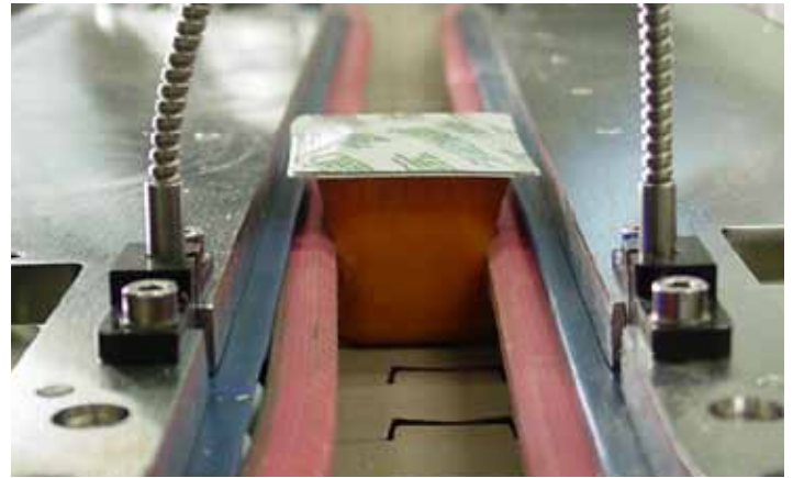
View of sample in the Dual Sensor Compression LP system. Note the opposing low profile 12mm belts.
