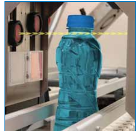
TapTone Fill_ir Sensor Close-up (Over fill detection, yellow arrows indicated point of inspection.)
